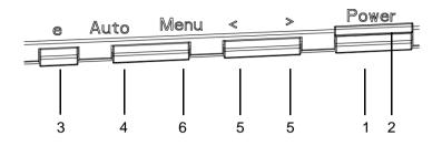
Front Panel Controls 1.Power Switch: To turn ON or OFF the power.
